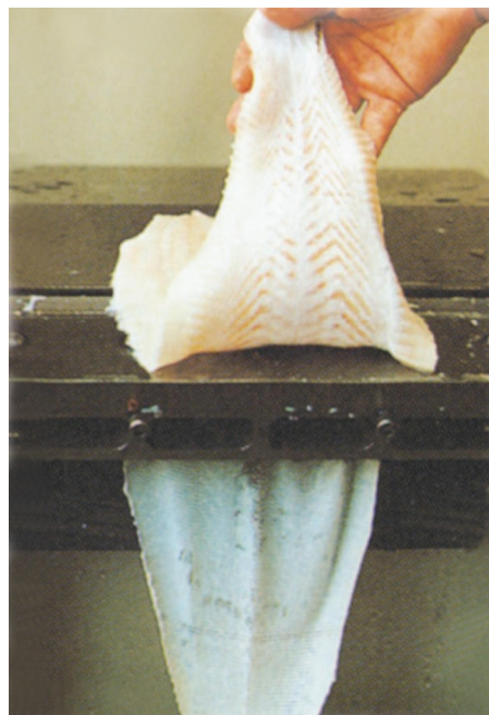
FIG. 2. A fish-skinning machine in action. Reproduced with the permission of Cretel NV, Gentsesteenweg, Belgium. Photograph kindly provided by Jerome Cretel of Cretel NV.
